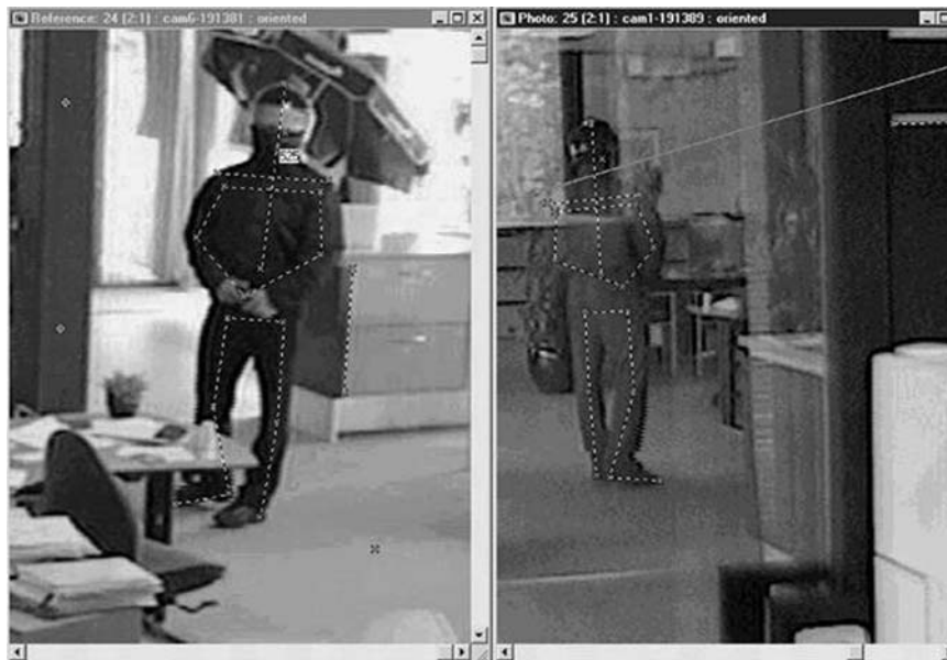
FIG. 5—Screen shot of Photomodeler Pro ® interface, showing selection of points. In the image on the left a point (“neck”) indicated by the label “525” has been selected. To select the similar point in the image on the right, which is from the other camera, the software shows the epilines (line of sight) as calculated from the first image. The point to be selected now must fall on this line, as well as being anatomically concordant with the first image.
